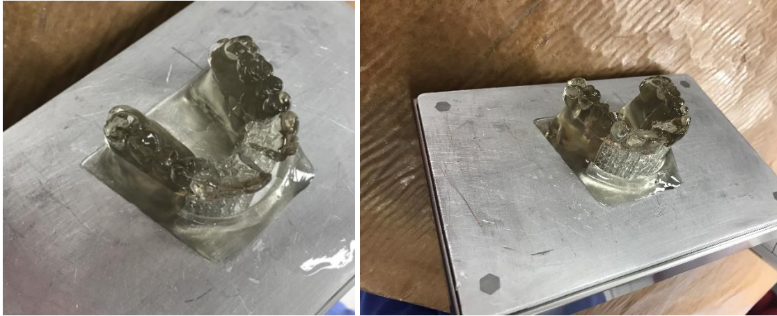
Figure 2.6: UR1 Test model on printer build plate prior to post processing.
